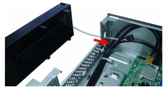
2. Connect the power button/LED cable to its mainboard connector.
